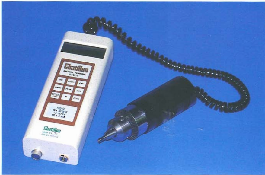
Figure 3—Chatillon Torque Gage consisting of the calibrated wrench attached to the control and display unit.
