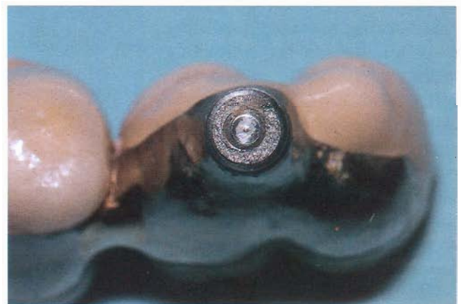
Figure 1D—Closer view of the fixture fracture surface. Fracture occurred at a level equivalent to the distal end of the abutment screw.
