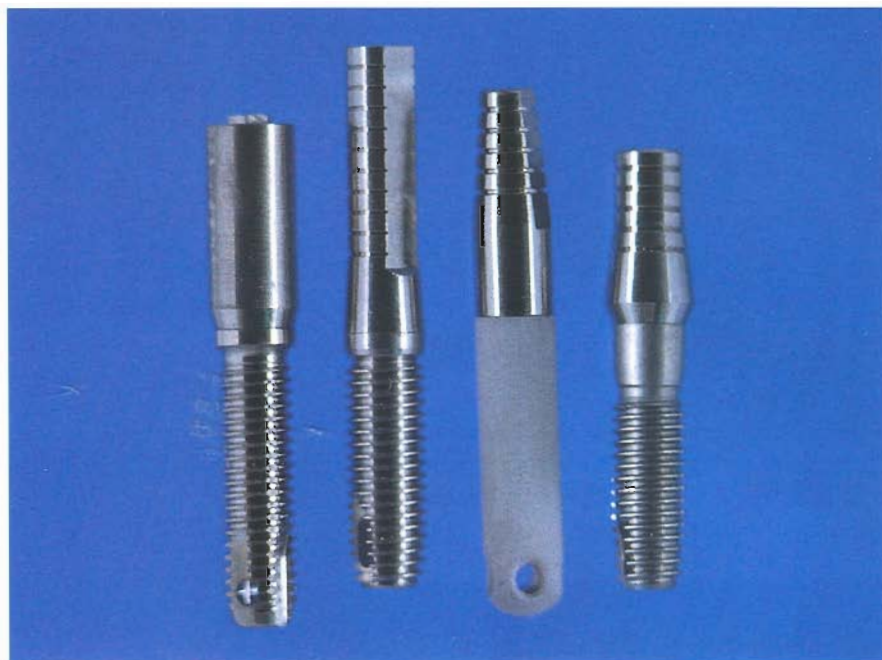
Figure 2—The four implant systems evaluated (shown from left to right): Nobelpharma, Dentsply Swede-Vent TL ® , Calcitek, and Dentsply Screw-Vent ® .
