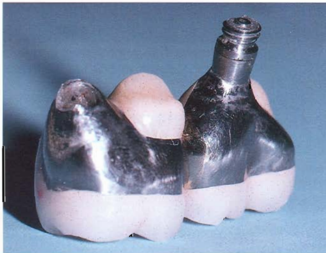
Figure 1C—Bridge removed from the mouth after fracture of the fixture below the premolars.
